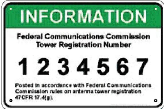
B | FCC REGISTRATION SIGN 8" HIGH X 12" WIDE WHITE/GREEN BACKGROUND, WHITE/BLACK LETTERING MOUNTING LOCATION: RIGHT GATE & BASE OF TOWER QUANTITY: 2
