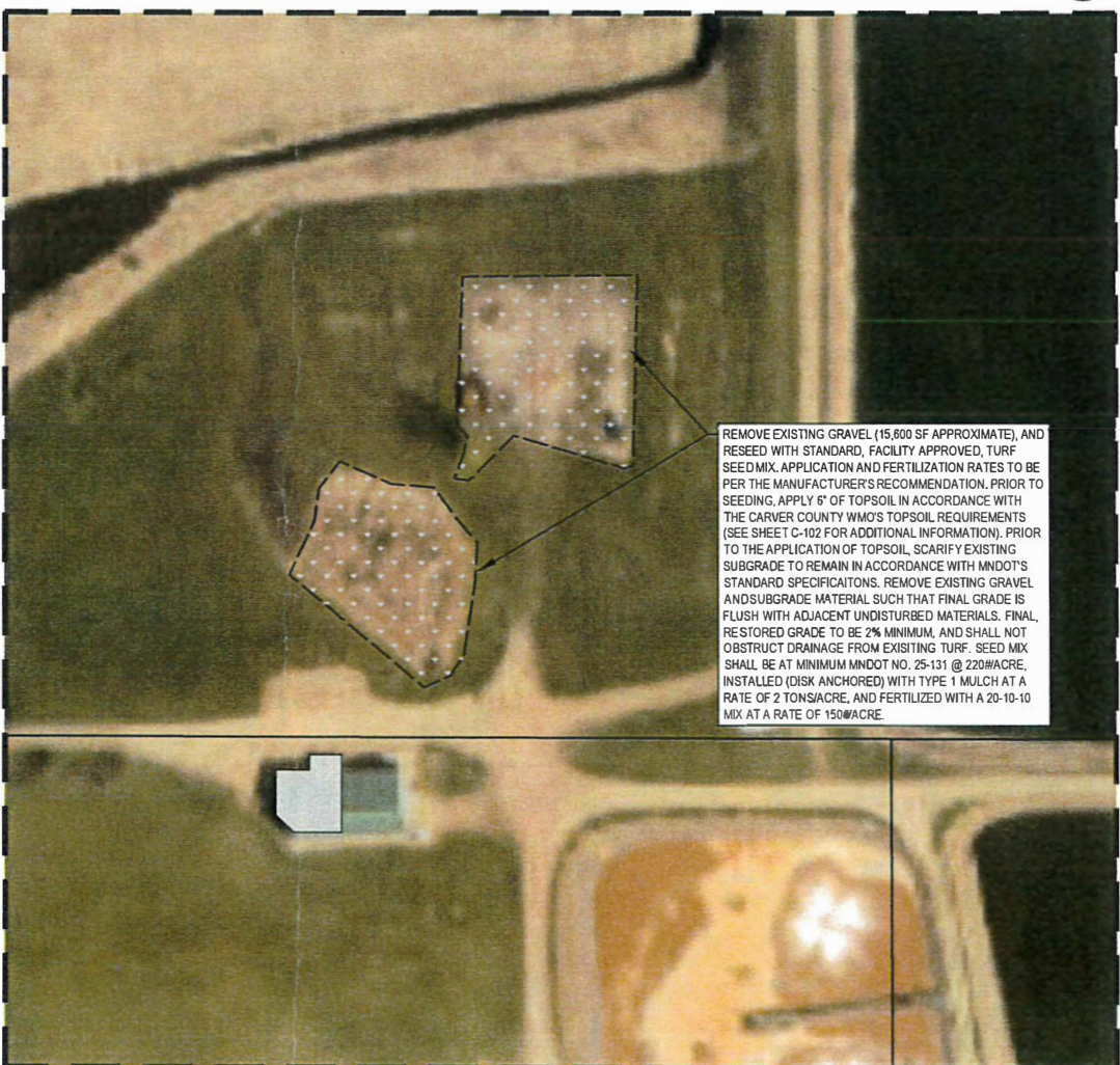
3 EXISTING GRAVEL DEMOLITION AND RESTORATION SCALE: 1" = 50'
